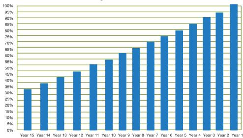
Proper maintenance can help your unit last decades. On the flip-side, a neglected unit loses roughly 5% of its efficiency each year that it operates without upkeep. So that green machine you bought to stay cool could start to function like the most inefficient thing on the market, if you fail to perform regular unit maintenance.
